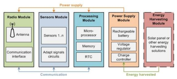
Fig. 2. Network device (node) architecture
